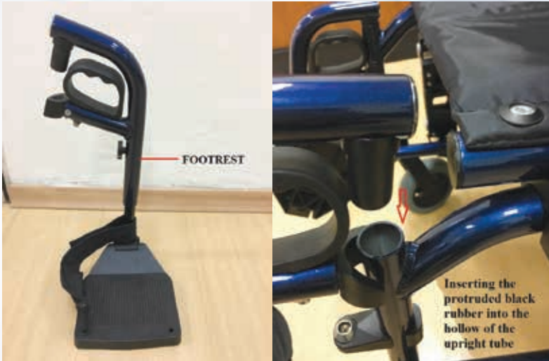
Figure 5. Footrest with Footplate (left), and Location for Attachment to the Wheelchair
